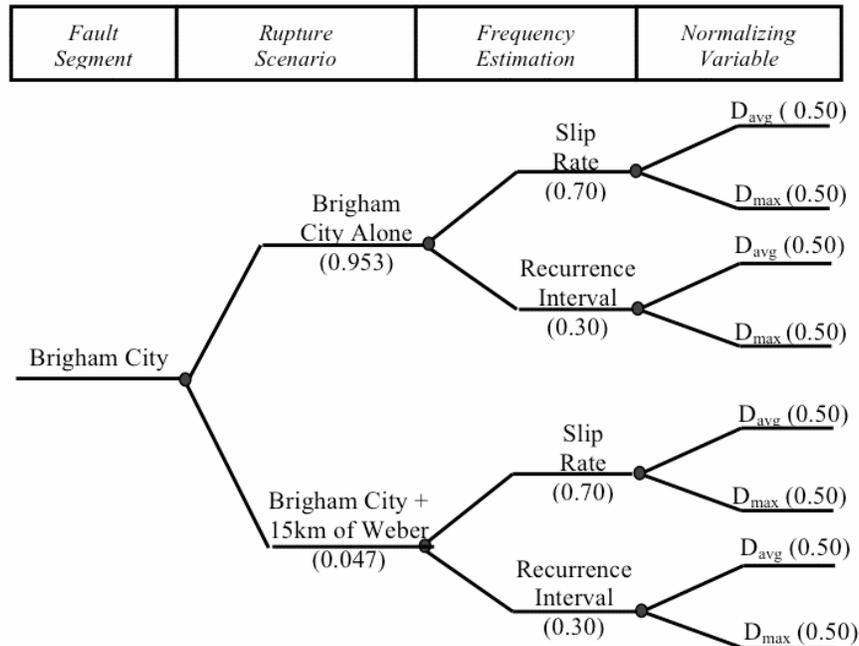
Figure 10. Brigham City segment branch of the Wasatch fault displacement hazard tree used for sample calculation.
