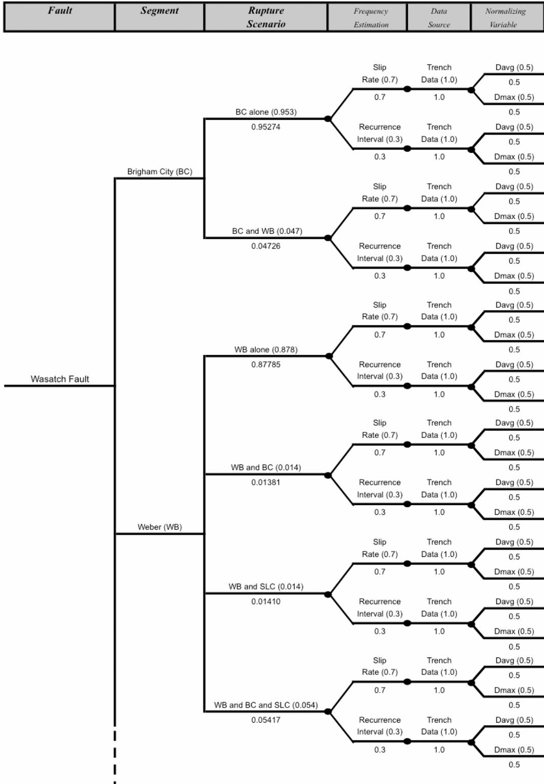
Figure 27. Detailed Wasatch Fault displacement hazard logic tree.
