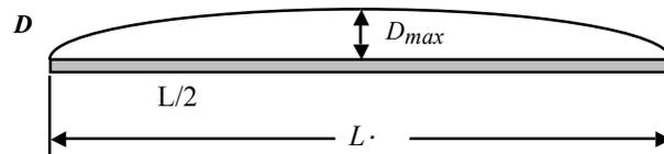
Figure 4. Cartoon illustration of elliptical fault displacement,  $D$ , distribution along fault length,  $L$ .
