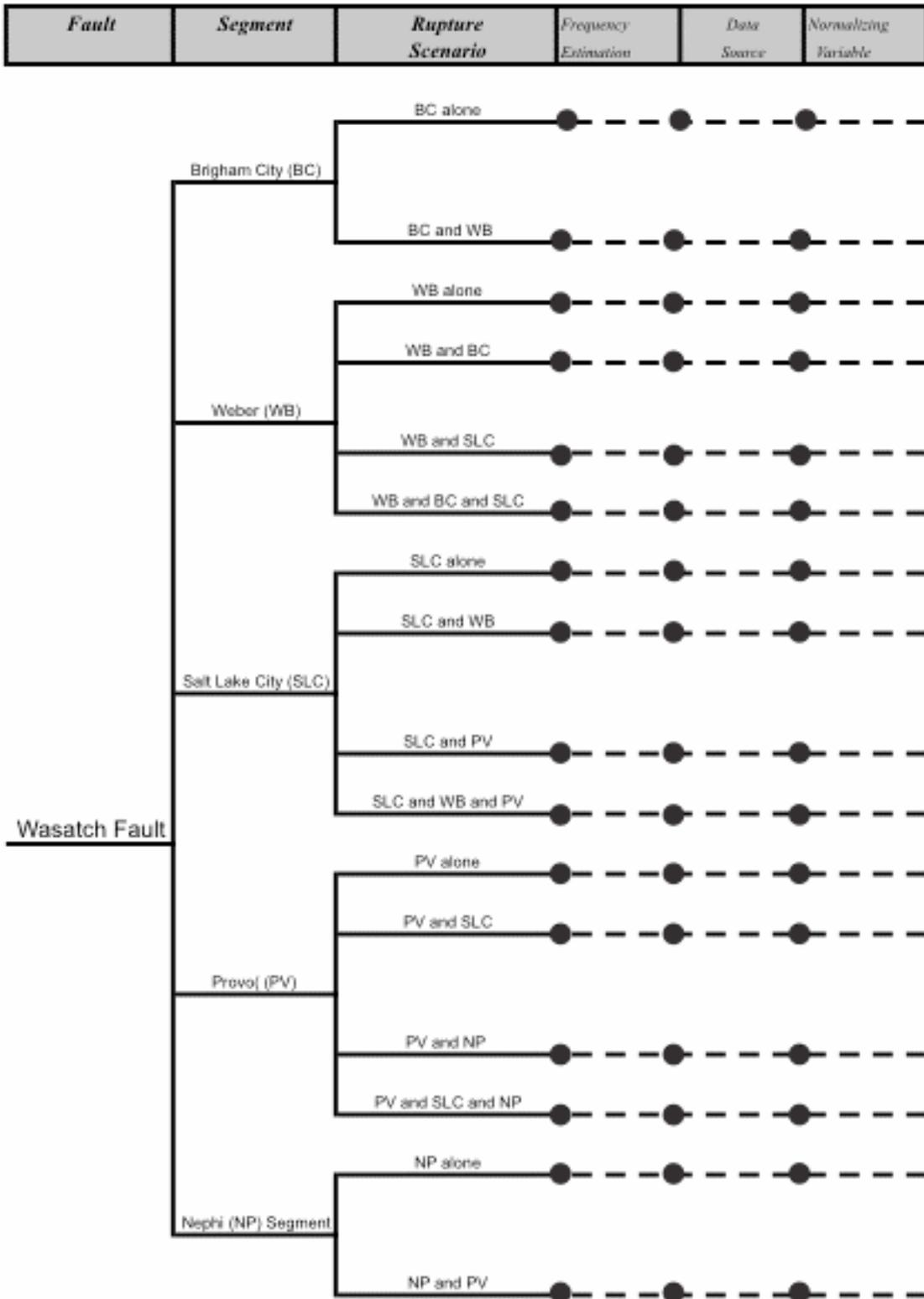
Figure 26. General layout for the Wasatch fault displacement hazard logic tree.
