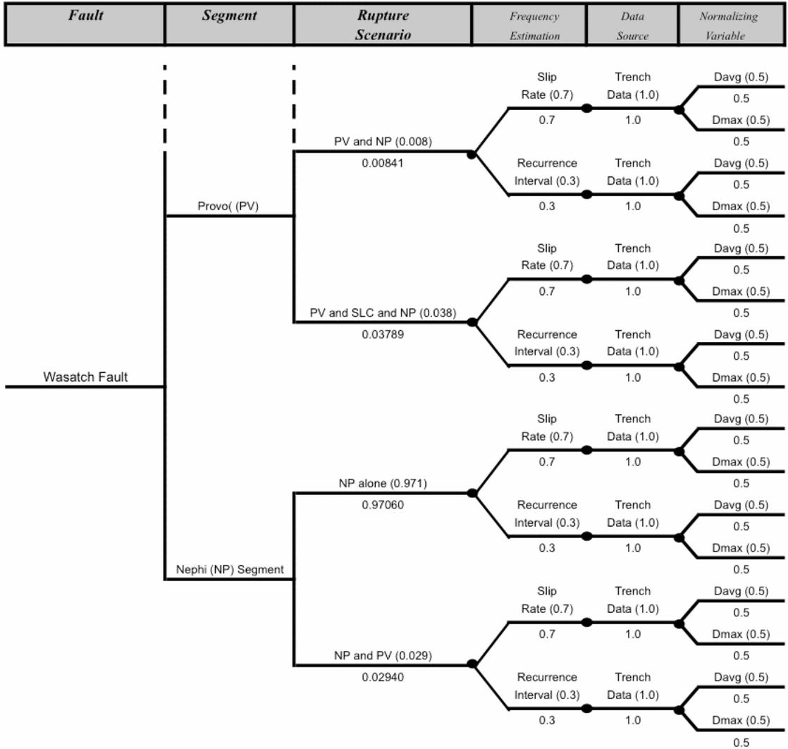
Figure 27. Detailed Wasatch Fault displacemant hazard logic tree *CONTINUED*
