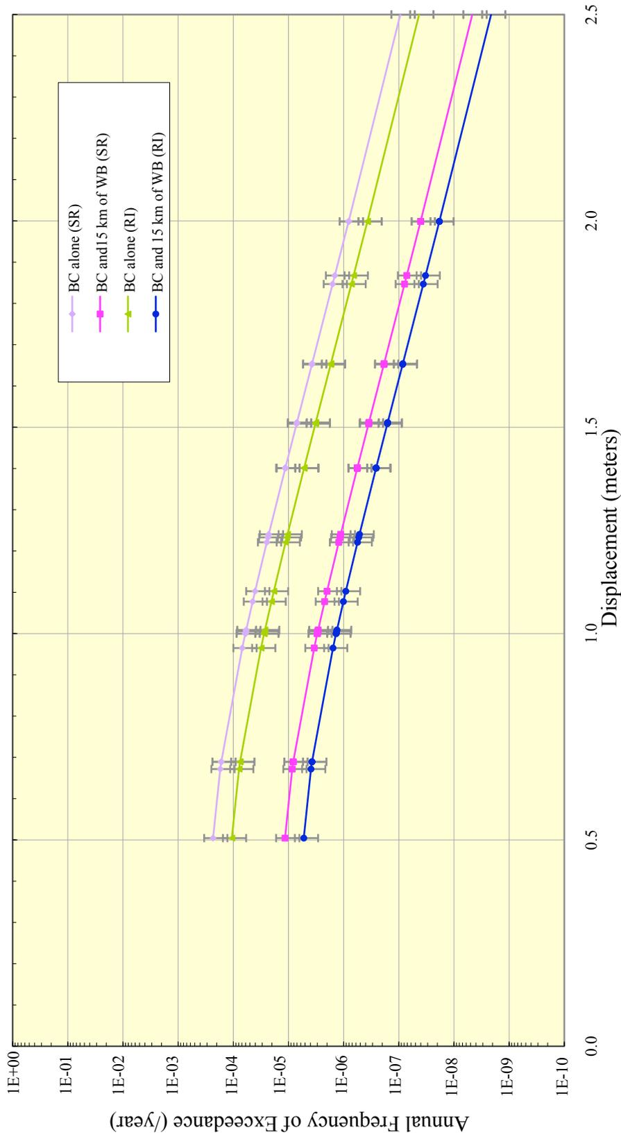
Figure 12. Brigham City segment hazard curves with  $D_{max}$  as the normalizing factor.  $D_{avg}$  for the segment is 1.2 meters and  $D_{max}$  for the segment is 1.7 meters. Abbreviations: BC = Brigham City Segment, WB = Weber Segment, SR = Slip Rate model used for frequency estimation, RI = Recurrence model used for frequency estimation. Uncertainty bands (5% and 95%) shown.
