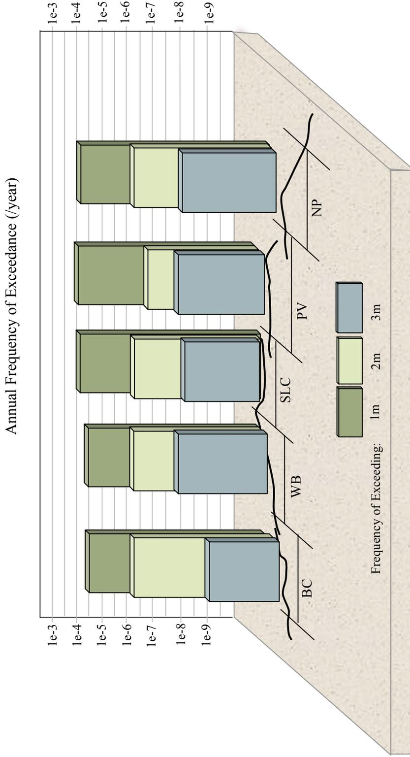
Figure 23. Comparative annual frequency of exceedign 1 meter, 2 meters, and 3 meters of displacement using single segment model, slip rate model, and  $D_{avg}$  as the normalizing factor. Abbreviations: BC=Brigham City Segment, WB=Weber Segment, SLC= Salt Lake City Segment, NP= Nephi segment, Pv= Prove Segment.
