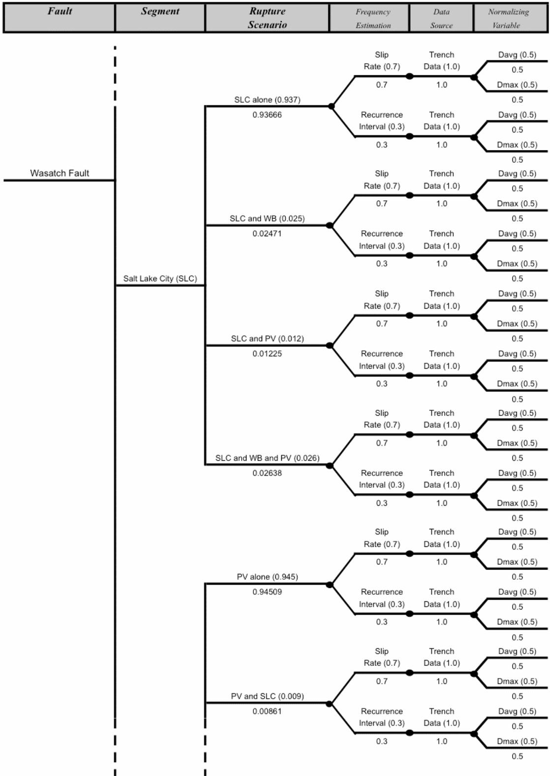
Figure 27. Detailed Wasatch Fault displacement hazard logic tree *CONTINUED*
