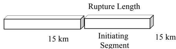
Figure 9. Cartoon illustration of multisegment rupture. Fault initiation on main segment and 15 kilometers of adjacent segment or segments.
